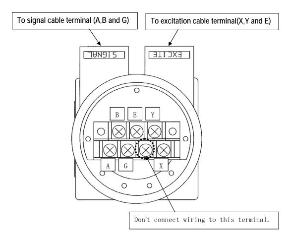
Figure 3.2.2 Terminal Block of GF632
